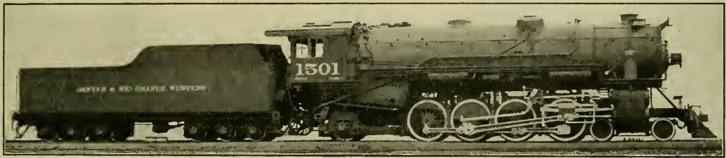
DENVER & RIO GRANDE RAILROAD MOUNTAIN TYPE LOCOMOTIVE. (BUILT BY THE AMERICAN LOCOMOTIVE CO.)
